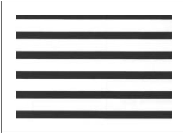
FIGURE 52: Background lines for viewing turbidity of a suspension in comparison to a turbidity standard
